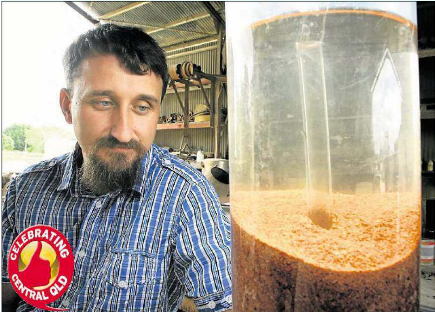
FILTRATION BREAKTHROUGH: Ben Kele says using volcanic rock to filter water could reduce the salt content by up to 40%.
