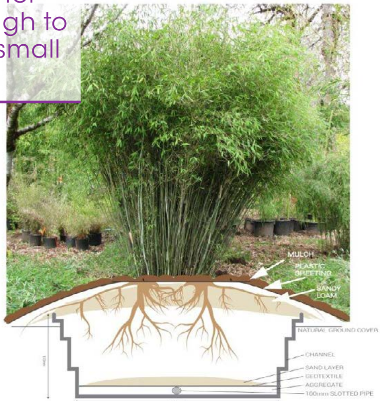
FIGURE 1 HOW THE RHIZOPOD WORKS ABOVE AND BELOW GROUND
